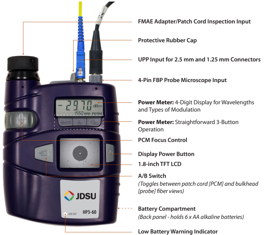
Inspect the Patch Cord with Integrated PCM and the Bulkhead with Probe
